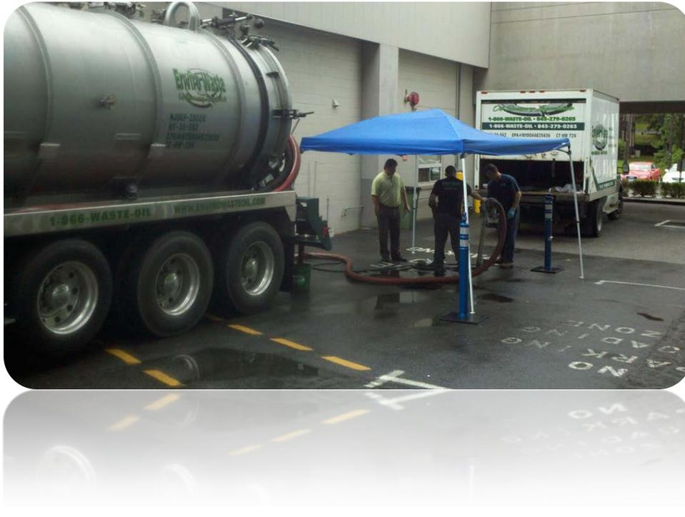
**Servicing & Maintenance.** Oil water separators (OWS) can be costly to maintain if not properly managed, and can be very expensive conduits of pollution. When cleaning is required, it should be performed by an experienced HAZWOPPER and OSHA certified OWS Maintenance Company.
